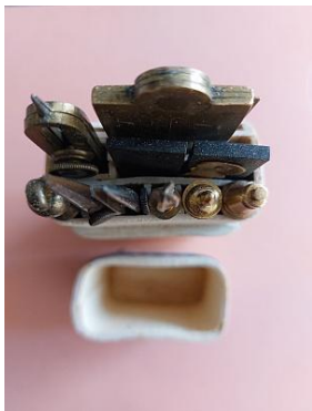
Positioning of the instruments, covering of the outside of the new case, both cases seen from above.
