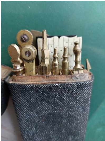
Pocket case with mathematical instruments for drawing mathematical figures. Around 1800.
