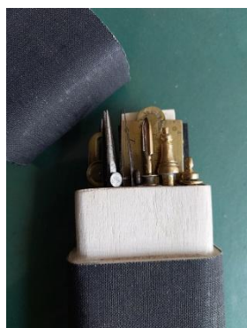
Positioning of the instruments, covering of the outside of the new case, both cases seen from above.
